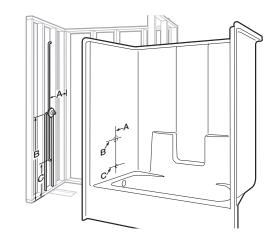
If mounting fittings — from stable reference points (back wall studs, floor) measure the locations of spout and valves. Note measurements below. For showers, refer to Diagram 2A; for tub-showers, refer to Diagram 2B.
