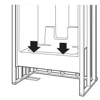
Place the unit into framing with drain fitting over and onto waste pipe with skirt firmly on the floor.
