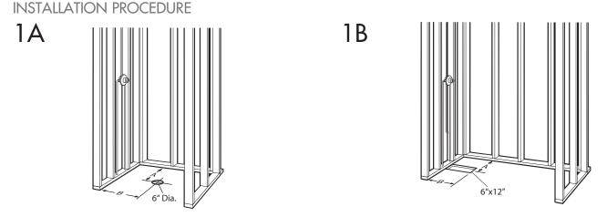
Note: If fire-rated alcove is required, approved finish material must be in place prior to unit installation to meet fire safety requirements of local building codes and/or FHA/HUD Minimum Property Standards.
