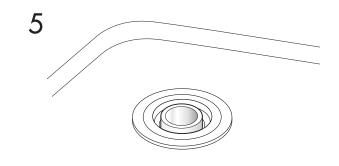
Assure waste pipe protrudes well into drain fitting. Maintain proper floor slope towards drain.
