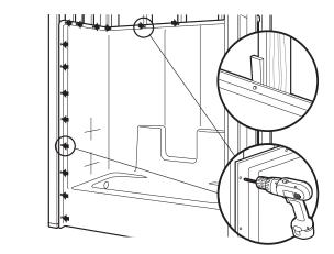
Pre-drill pilot holes. Fasten panel to framing at every stud and eight inches vertically through nailing flange.
