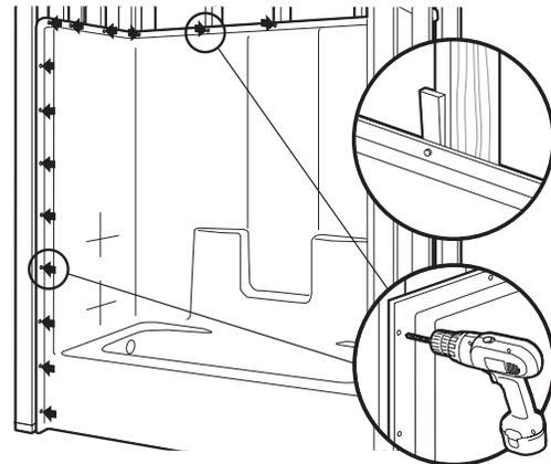
Pre-drill pilot holes. Fasten panel to framing at every stud and eight inches vertically through nailing flange.
