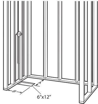
Note: If fire-rated alcove is required, approved finish material must be in place prior to unit installation to meet fire safety requirements of local building codes and/or FHA/HUD Minimum Property Standards.
