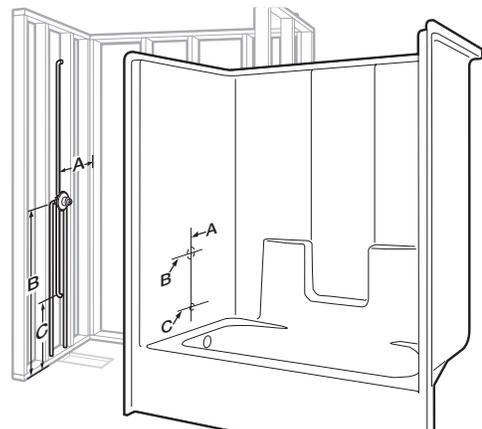
If mounting fittings — from stable reference points (back wall studs, floor) measure the locations of spout and valves. Note measurements below.
