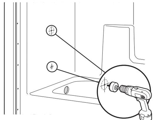
Mark fitting locations. (Refer to measurements from step 2.) Using a hole saw (fine tooth or abrasive grit cutting edge), make necessary openings for filler and valves, drilling from inside (smooth side) out.
