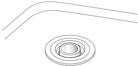
Assure waste pipe protrudes well into drain fitting. Maintain proper floor slope towards drain.
